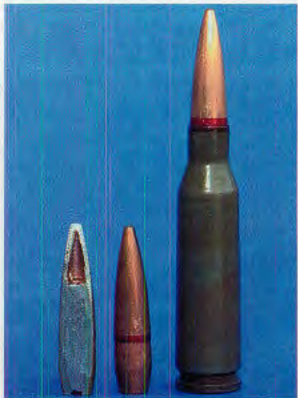
A mystery round in the 1980s, Wolf Performance Ammunition offers 5.45x39 ammunition to the American shooter. Featuring a 60 gr. FMJBT with an airpocket in the nose, it averaged 2,954 fps across the chrony.
